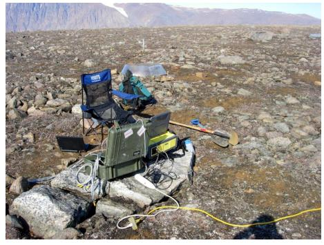
Gasmet DX4015 used for greenhouse gas monitoring. Photo by Martin Brummell
