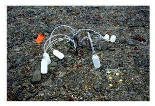
equilibrium via diffusion over 24 hours. This allowed the researchers to analyse gas concentrations to a depth of 0.5 metre. The procedure was simple and therefore reliably repeatable.
