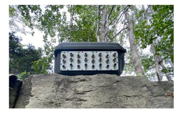
The eosMX is a portable, weather resistant recirculating multiplexer that offers unmatched flexibility for automating coordinated gas sampling in a lab or field setting. Choose between 8 or 16 sampling ports and connect up to 4 eosMX units to sample from up to 64 locations using a single gas analyzer.
